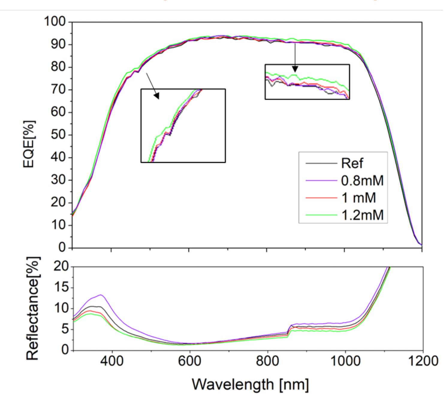
➤ Si nanopyramids fabricated by AgNO<sub>3</sub>-assisted alkaline etching method exceeding the EQE of that of industry-standard Si solar cells.
