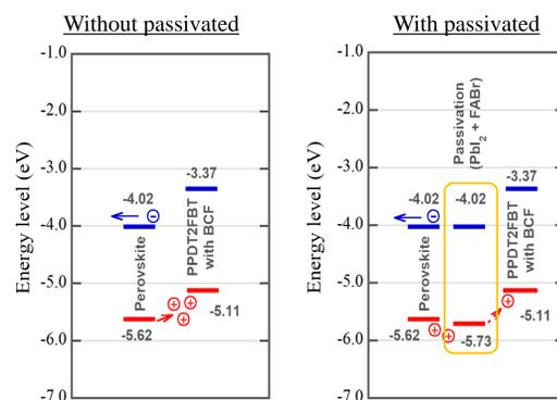
The carrier recombination was suppressed by inserting the passivation layer.
