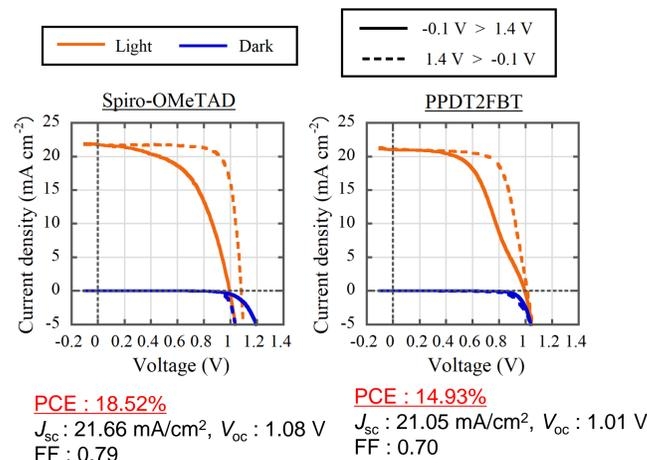
The PCE of PPDT2FBT based devices decreased compare to that of standard PSCs with spiro-OMeTAD.
