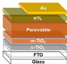
Fig. 4 Device structure.
