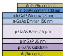
Schematic and details of GaAs 1J
