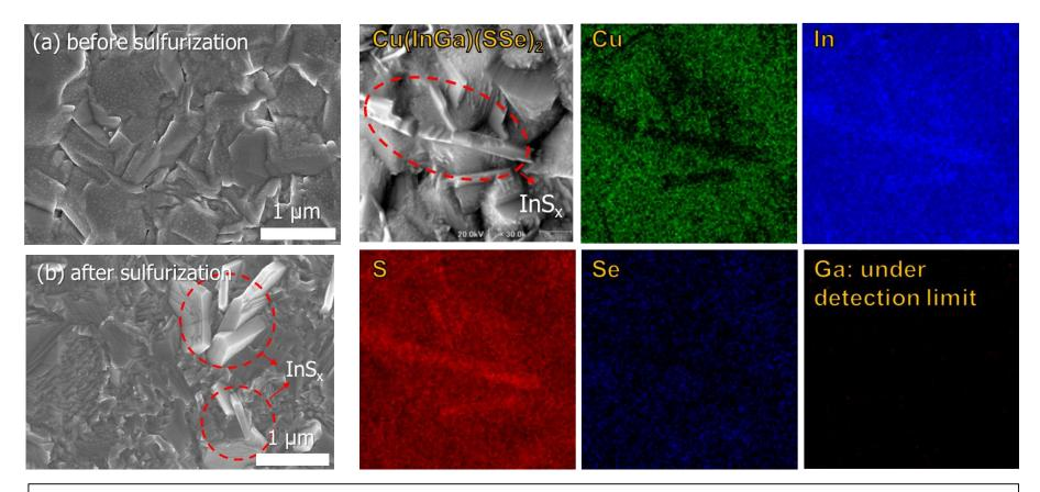
✓ After sulfurization Ga was not detected at the surface sulfurized CIGSe.
