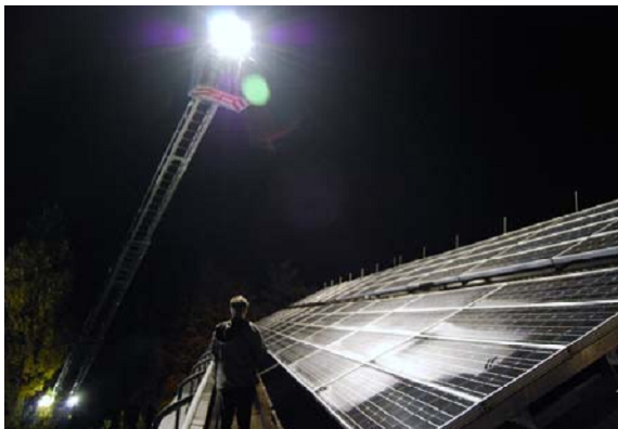
Fig. 1: Situation at the PV generator of sub-plant West of the PV test plant of BFH-TI under illumination by two floodlights of 1 kW on Oct. 27 th , 2010 by the fire brigade of the town of Burgdorf (minimum distance 7 m).
