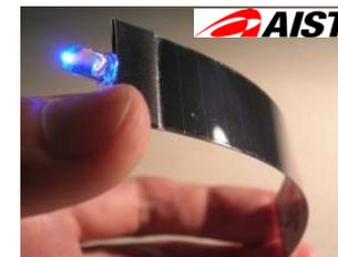
Monolithically integrated flexible CIGS mini-module
