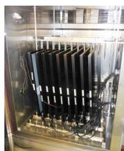
Chamber for test with forward bias
