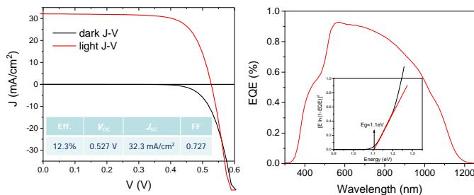
The highest efficiency of Ge incorporated kesterite solar cell greater than 12% [4]
