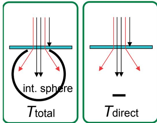
$$\text{Haze} = \frac{T_{\text{total}} - T_{\text{direct}}}{T_{\text{total}}}$$
