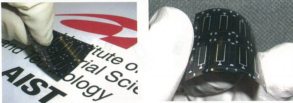
flexible CIGS solar cells on ceramics \eta=17.7\% (left) , Ti-foil \eta=17.4\% (right) and polyimide \eta=14.7\%
