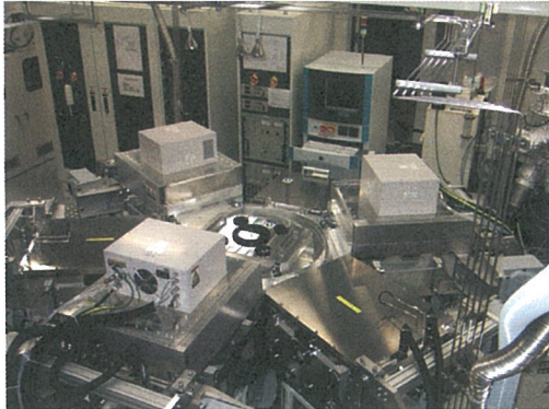
310 mm × 410 mm基板対応 薄膜シリコン太陽電池用プラズマCVD装置 Plasma CVD apparatus for thin-film silicon solar cells with a substrate size of 310 mm × 410 mm.
