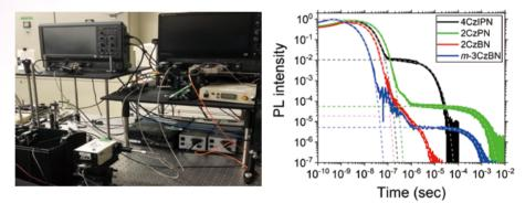
Photograph of transient photoluminescence apparatus (left) and an example of transient photoluminescence time profile (right)
