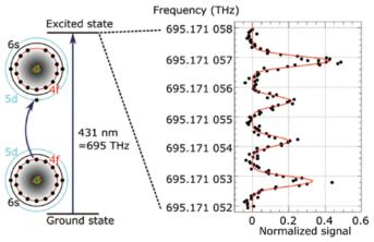
Change in the electronic structure of the observed transition and spectrum of the transition for the F = 3/2 hyperfine transition level
