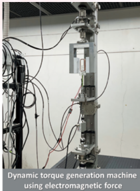
Measurement of dynamic torque generated by dynamic torque generation machine.
