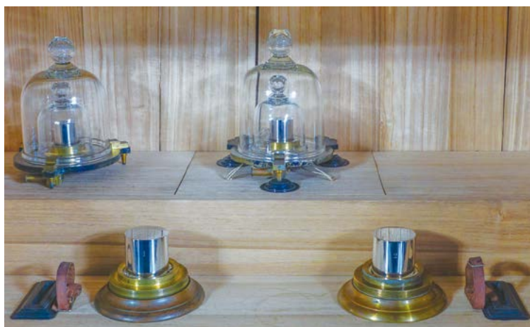
Upper center: National Prototype of the Kilogram of Japan Upper left: Secondary Prototype of the Kilogram Lower left and right: Prototypes of the Kan
