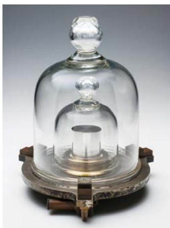
National Prototype of the Kilogram of Japan which was used as the national mass standard for about 130 years.
