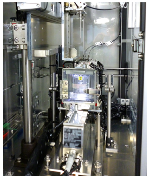
Gravimetric system using high-speed switching valves for calibration of low fuel flow rate.
