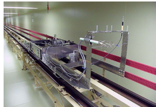
Primary standard for low air speed
