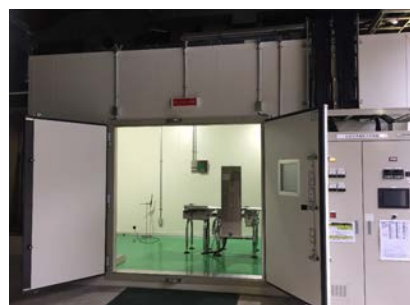
Figure 1: Temperature & humidity test chamber for static temperature & dump heat test 4.5 m (W) × 2.7 m (D) × 2.5 m (H)
