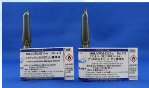
CRMs for doping test (standard solutions of 4-hydroxy-clomifene, left, and 3β, 4α-dihydroxy-5α-androstan-17-one, right)
