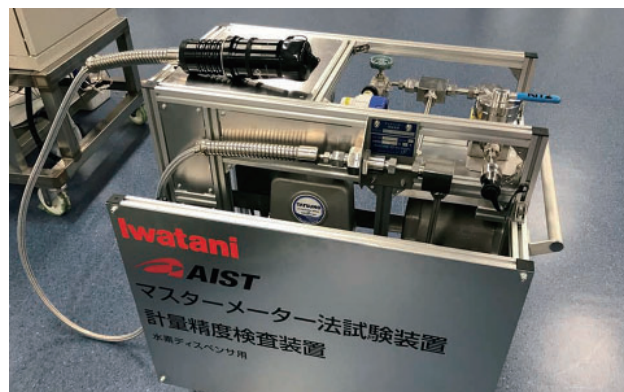
Figure 2: Test equipment of measurement precision of hydrogen dispenser with a master meter method.
