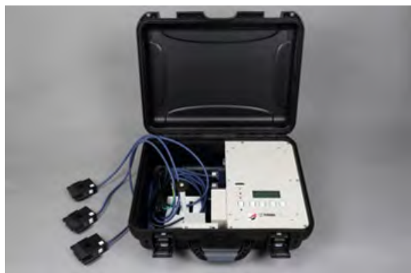
Photograph of developed portable high-precision DC current meter with clamp type DC current sensors
