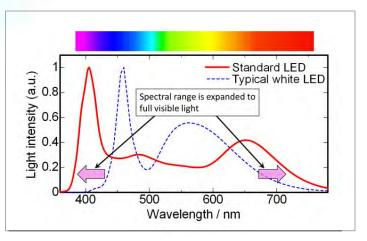
Spectra of the developed standard LED and a typical white LED
