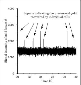
An example of analytical results of the goldrecovered *G. sulphuraria* cells from metal wastewater by using NMIJ originally-developed single-cell elemental analysis system.
