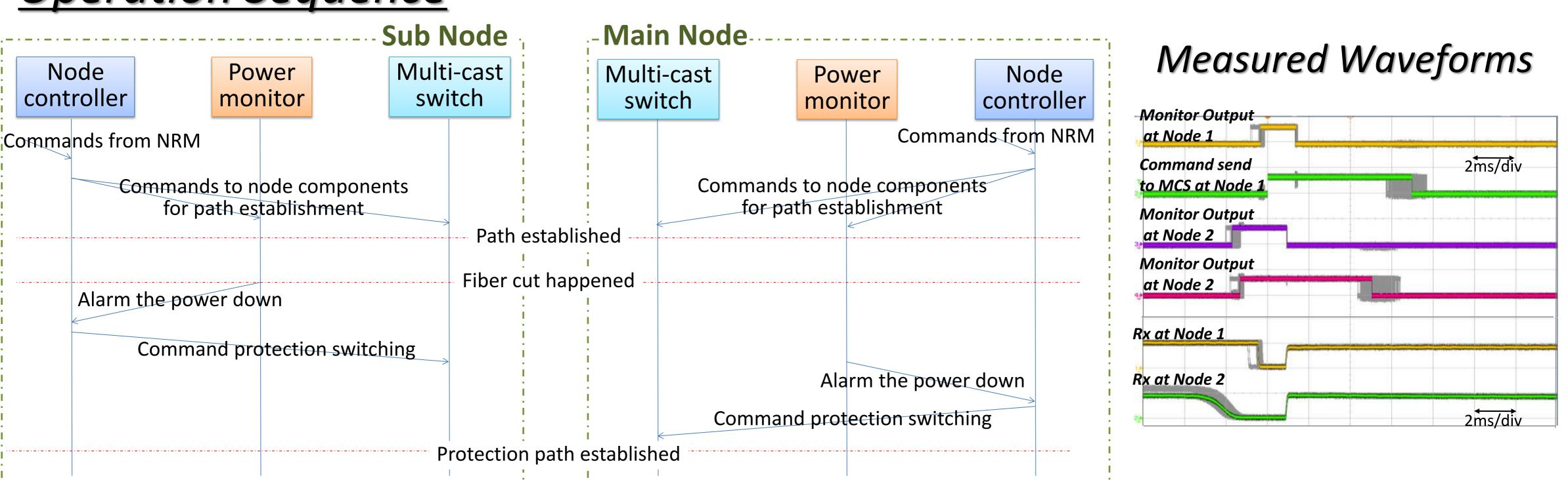
A node controller is the key to robustly realize disaggregated optical node platforms. The node controller aggregates node components and eases the operations of NMS.
