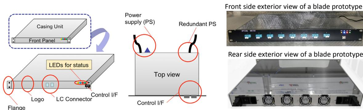
**Fig. 4:** Blade configuration diagram and prototype pictures
