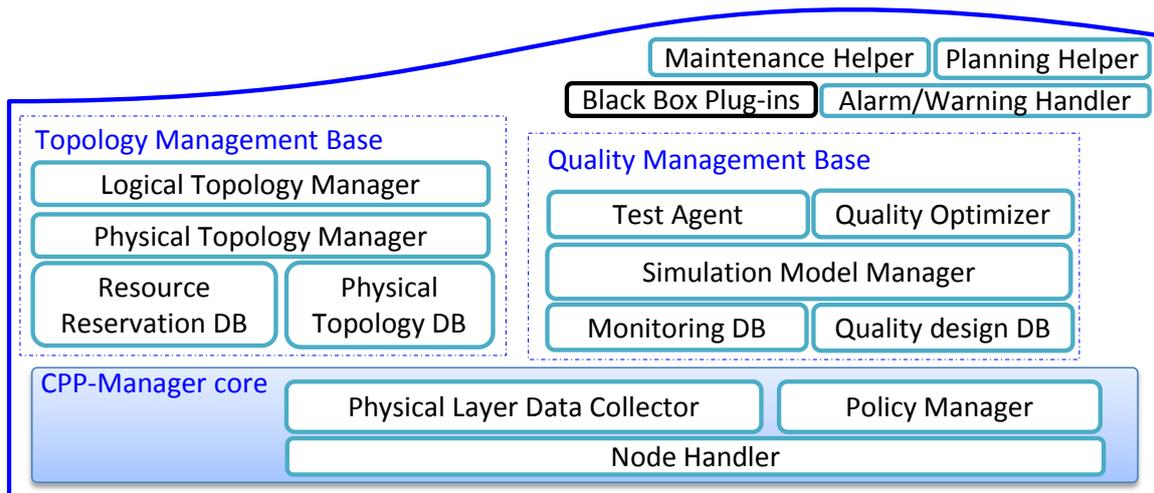
Fig. 2: Software architecture of CPP-Manager
