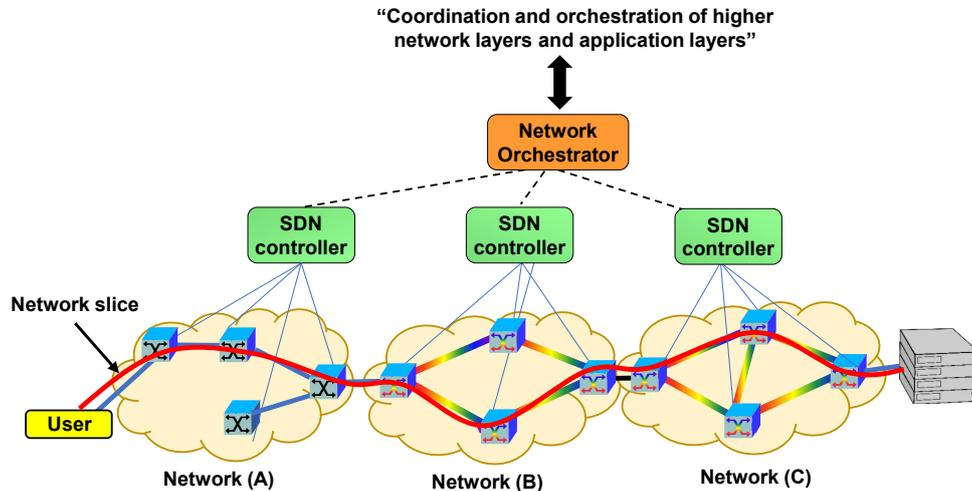
Fig. 7: Concept of network orchestration in the optical layer
