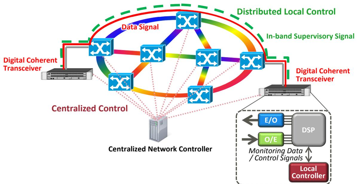
**Fig. 10:** Autonomous local control for optimal operations under the supervision of the centralized network controller
