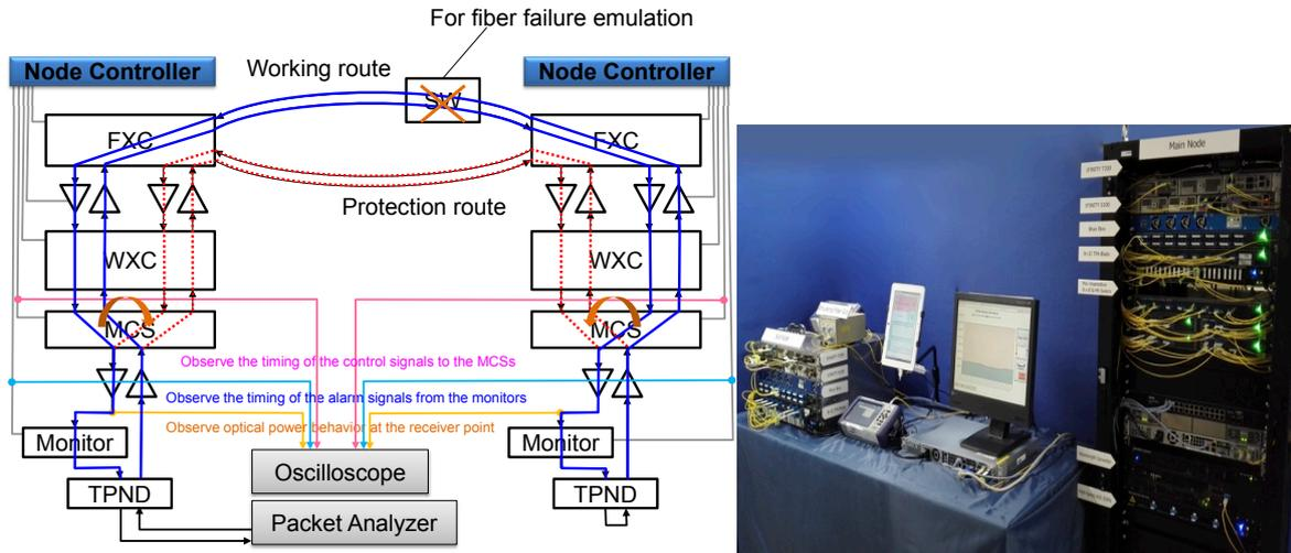
Fig. 11: Inter-blade cooperation for fast protection
