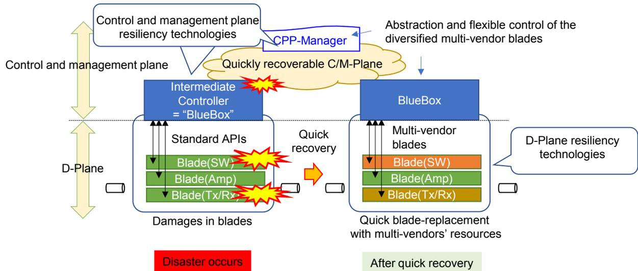
Fig. 8: Enhanced resilience with CPP technologies (in disaster recovery)
