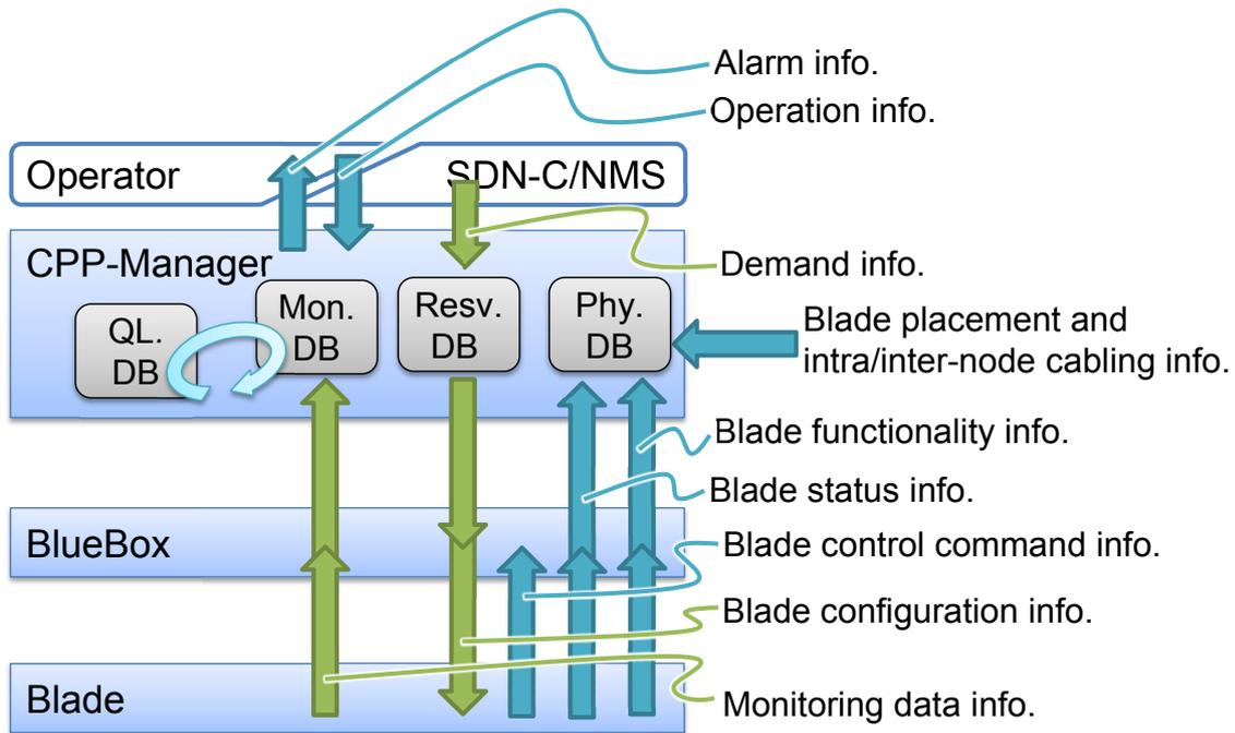
**Fig. 5:** Overview of the flow of the exchanged information; the green arrows denote dynamic path provisioning/deletion and the blue arrows denote installation or maintenance cycles.
