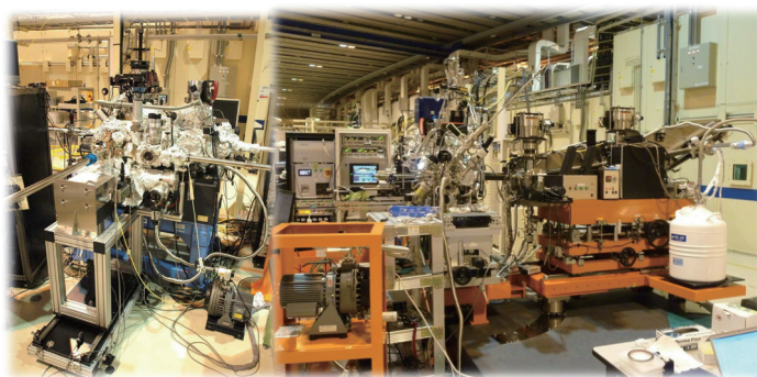
Figure 1 Angle-resolved high-resolution soft X-ray photoelectron spectroscopy system and soft X-ray emission spectrometer
