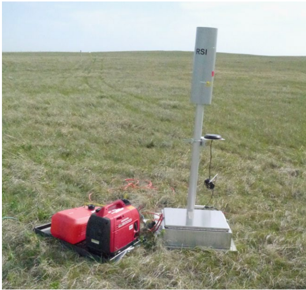
Nal-scintillator-based environmental monitor (ICRU Report 92)
