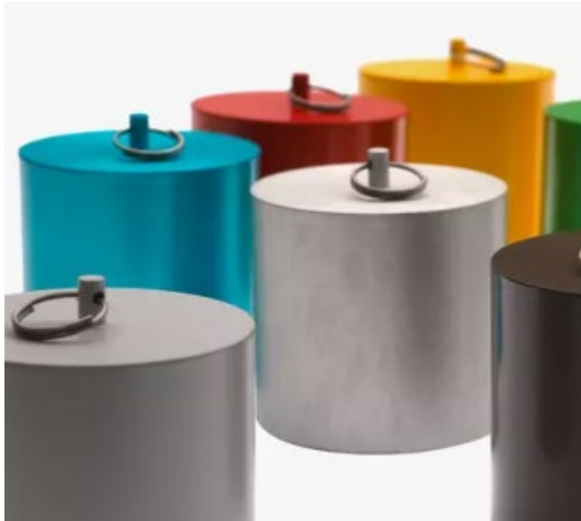
“Seibersdorf” cylinder 6 cm Ø x 6 cm, PMMA 1 or 2 Harshaw TLD cards
