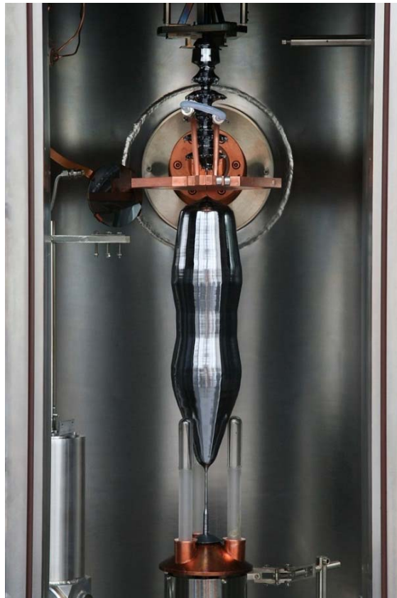
Avo28 grown by the float-zoning method at IKZ (May 2007)
