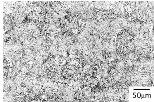
Fig.16 Microstructure of C3(Fe-0.3mass%C) ( Optical microscope image )
