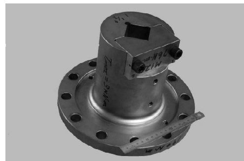
Fig. 4. Square hole adapter flange (nominal size: 38 mm) used in the 20-kN·m-DWTSM
