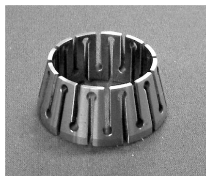
Photo 1 The metal collet for chucking outer cylinder (stainless steel).
