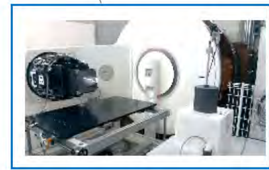
Photon fields with 6 MeV-7MeV using a medical LINAC
