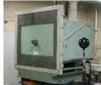
Parallel plate Free ionization chamber
