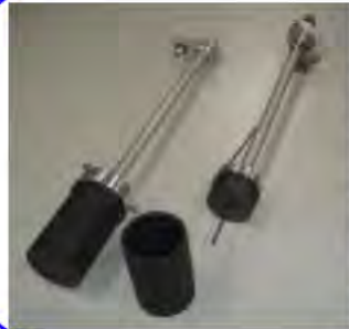
Graphite wall cavity ionization chamber
