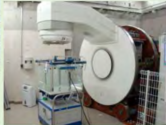
Co-60 146TBq Linac photons 6MV, 10MV, 15MV Linac electrons 9MV 12MV 15MV 18MV
