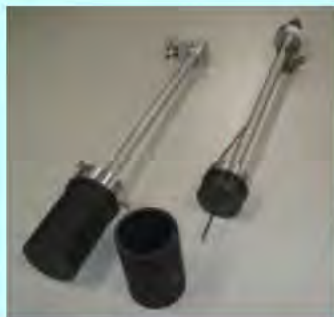
Graphite-walled cavity chamber
