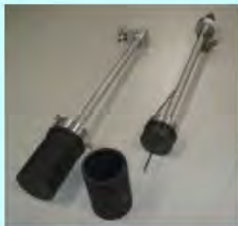
Graphite-walled cavity chamber
