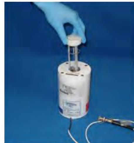
Well-type ionization chamber
