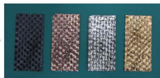
From left: Pre-plating, copper plating, nickel plating, and gold plating Carbon fiber epoxy resin prepreg (uncured) TR3110 381GAX (Mitsubishi Rayon)
