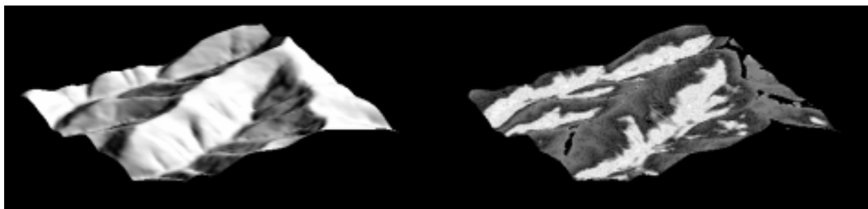
Figure D-1. Total radiance (radiosity) emitted from an isothermal homogeneous scene ( \epsilon=0.9 ), consisting of directly emitted and multiple-scattered components. Left: Digital elevation model "illuminated" by sun at lower right, assuming a Lambertian surface of uniform reflectivity. Right: Multiple-scattered TIR component, contoured with black = 0-1%, gray = 1-3%, and white = 3-5% of the direct emitted component. Perspective view calculated from a 7.5' DTM having horizontal resolution of 30 m. Subscene is 3 km across.
