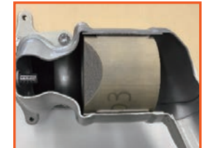
Nitrogen recycling & Catalytic conversion device (NO emission)
