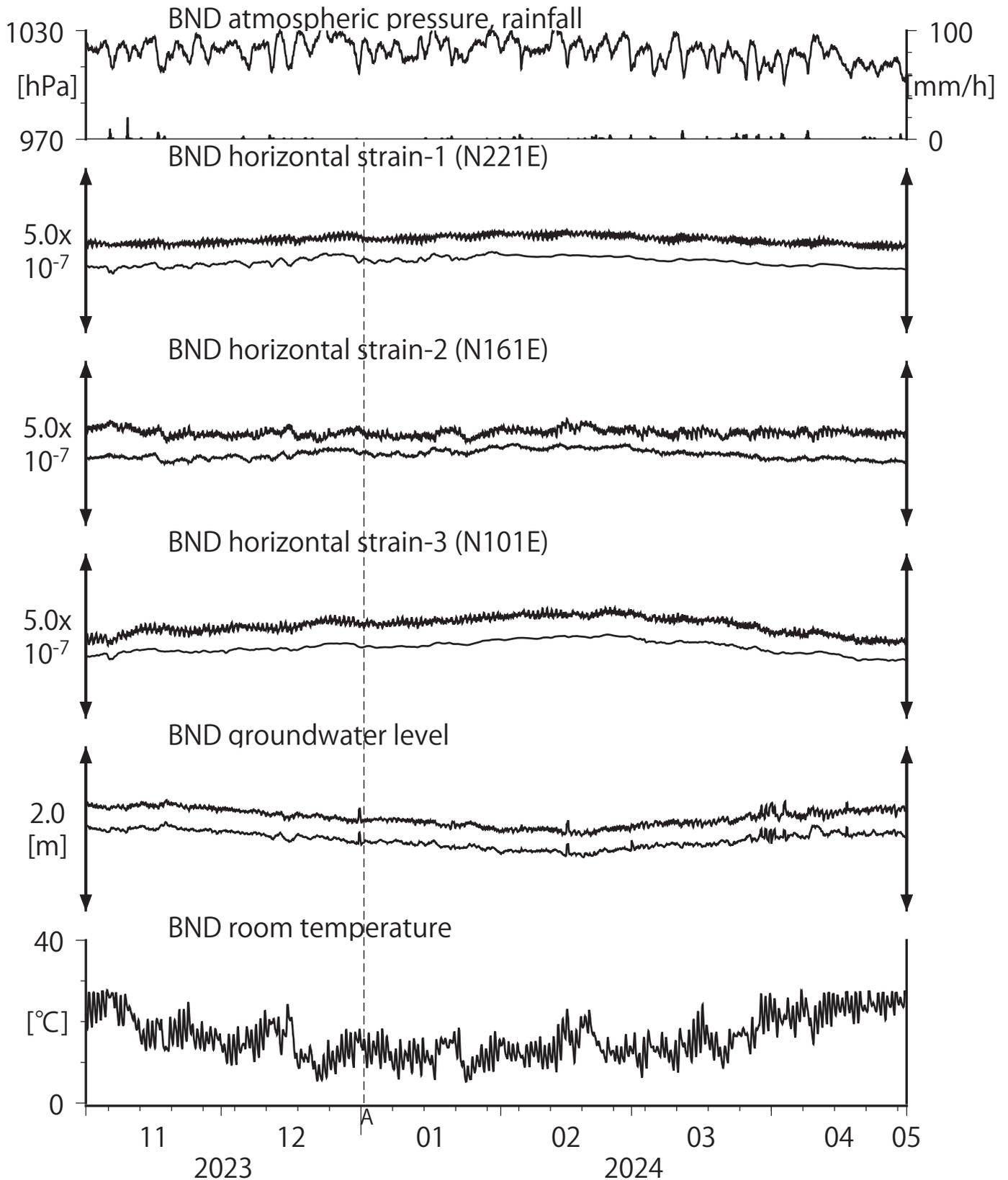
Strainmeter depth = 496.5-496.7 [GL-m]
