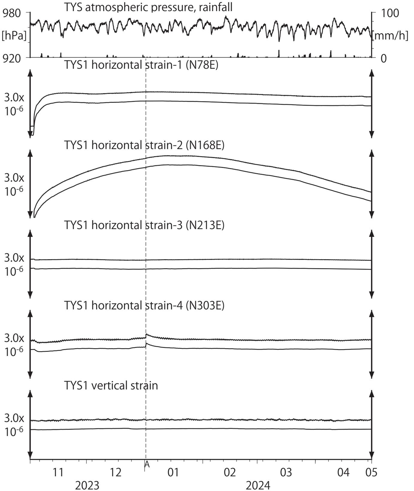
Strainmeter depth = 586.7-588.1 [GL-m]
