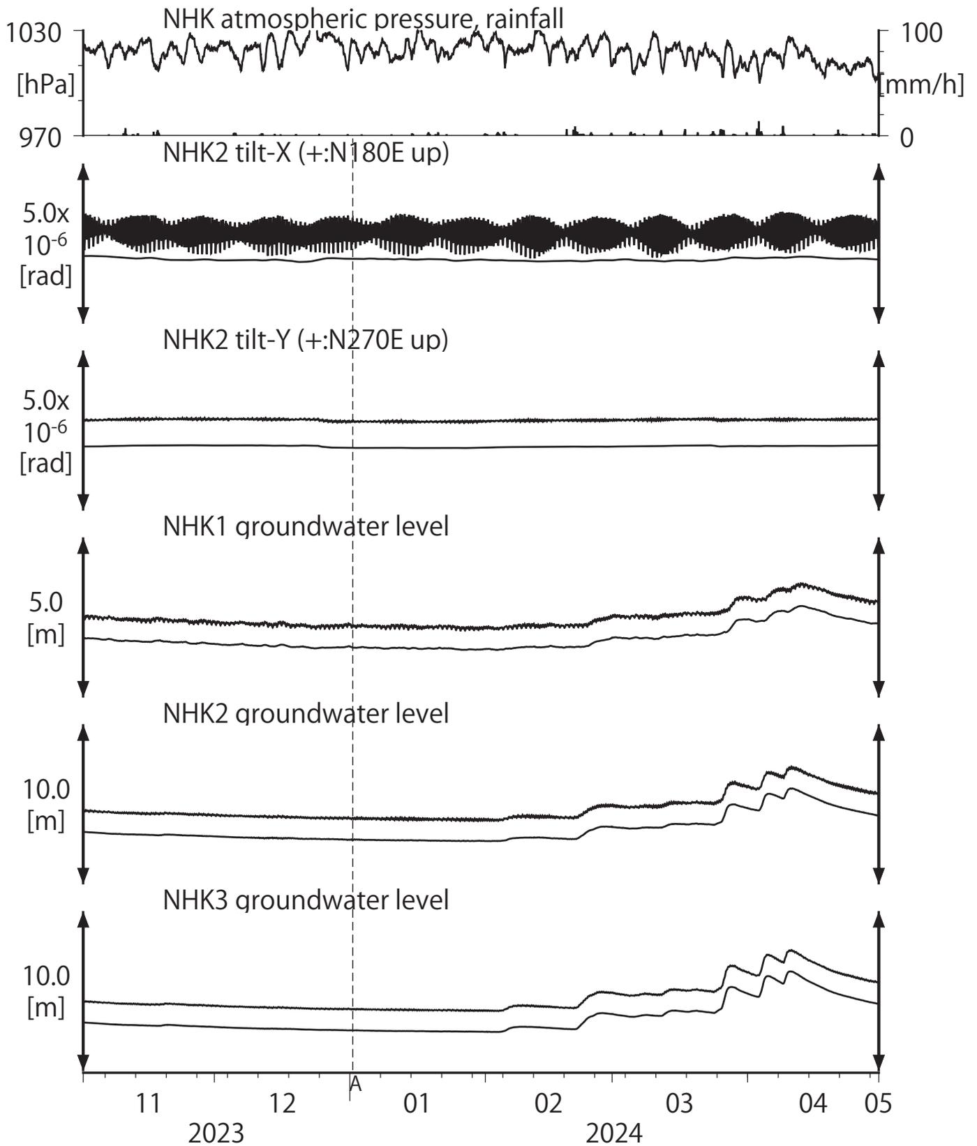
Tiltmeter depth = 196.7-197.3 [GL-m]
