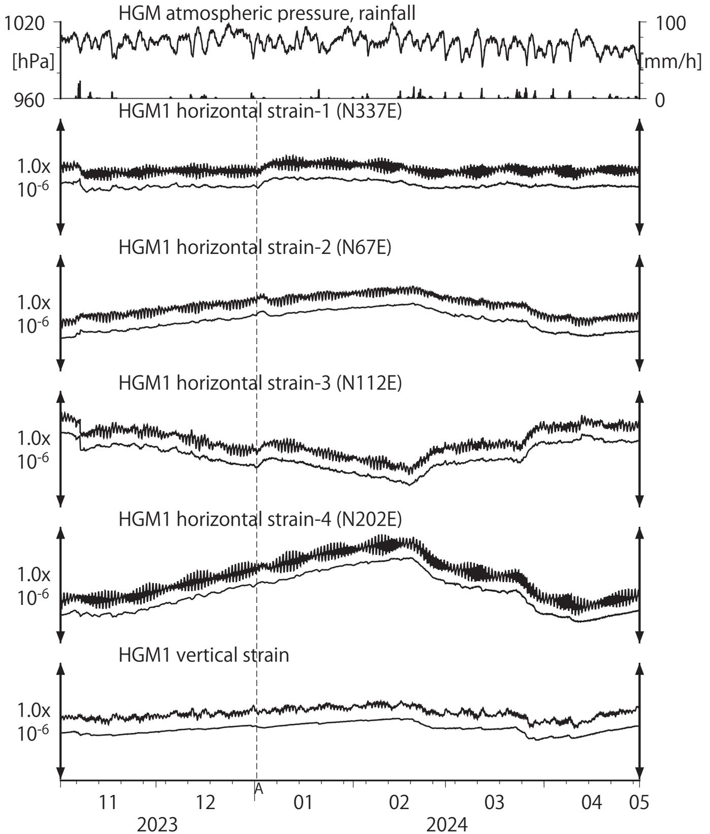
Strainmeter depth = 372.7-374.1 [GL-m]
