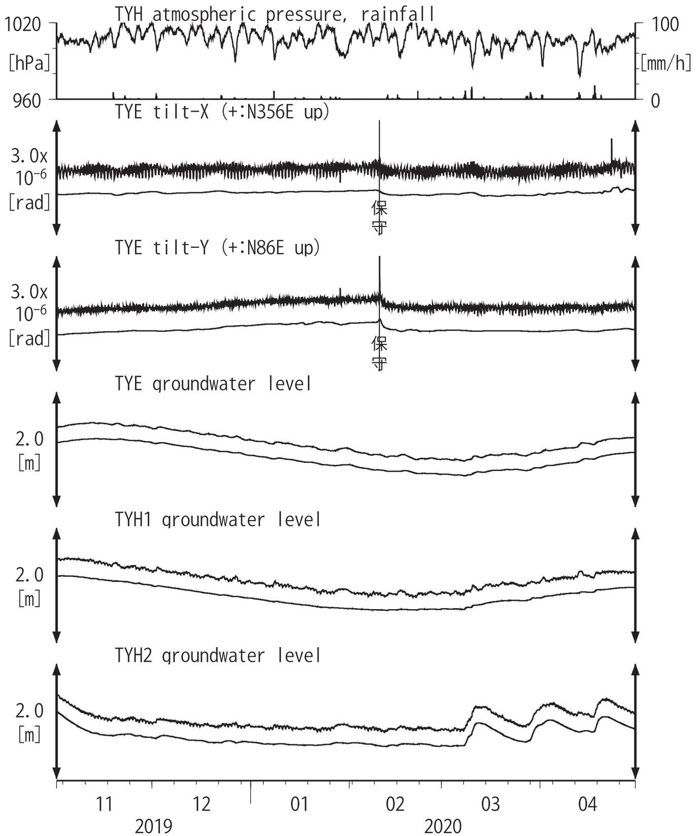
Tiltmeter depth = 265.6-266.5 [GL-m]
