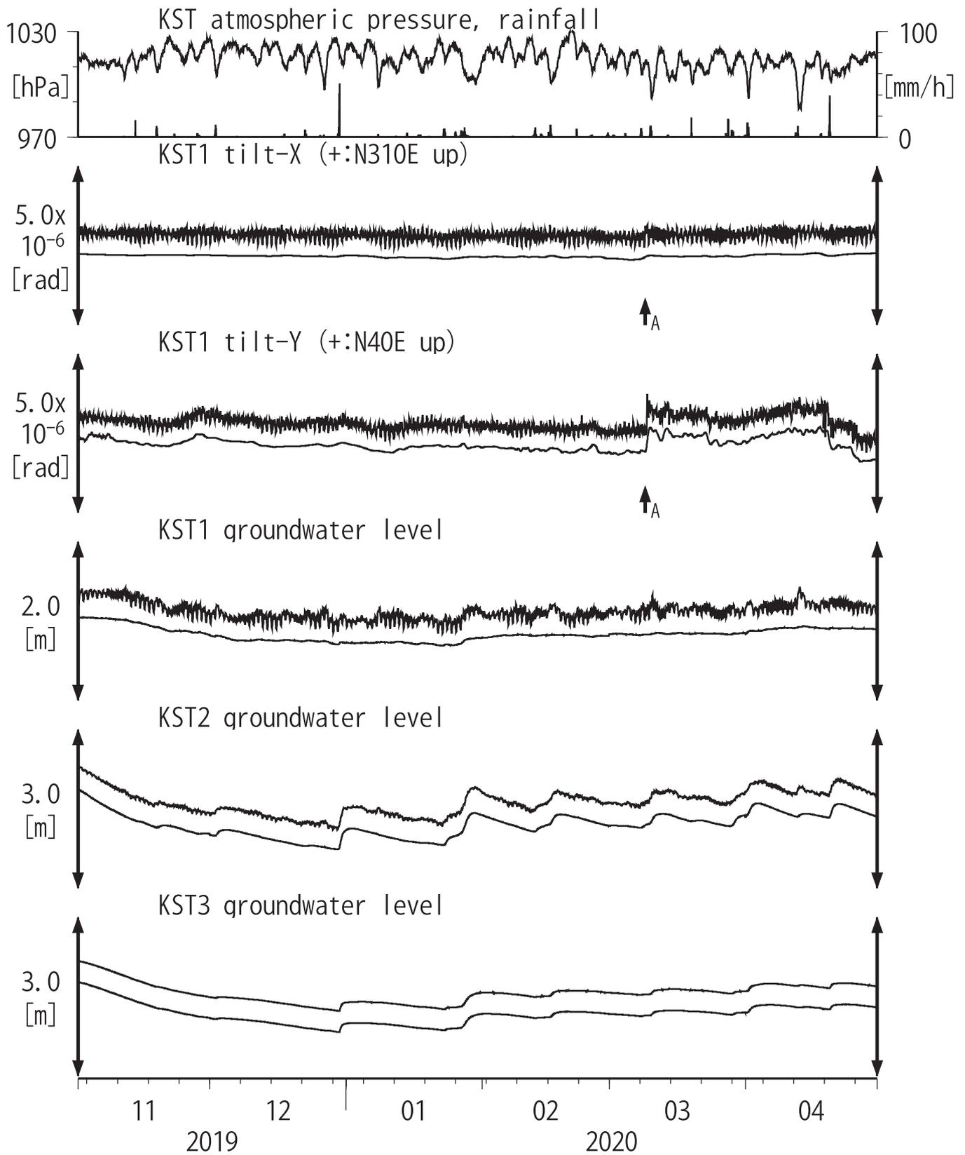
Tiltmeter depth = 589.0-589.8 [GL-m]
