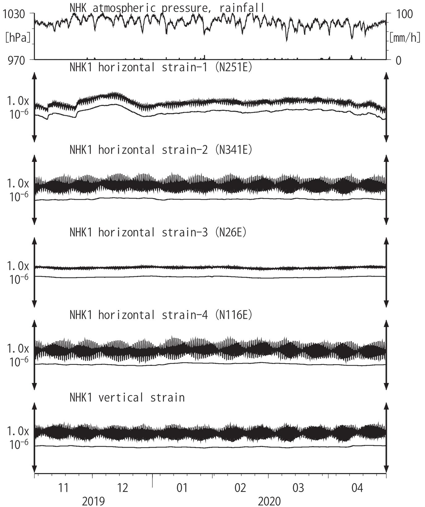
Strainmeter depth = 481.0-483.0 [GL-m]
