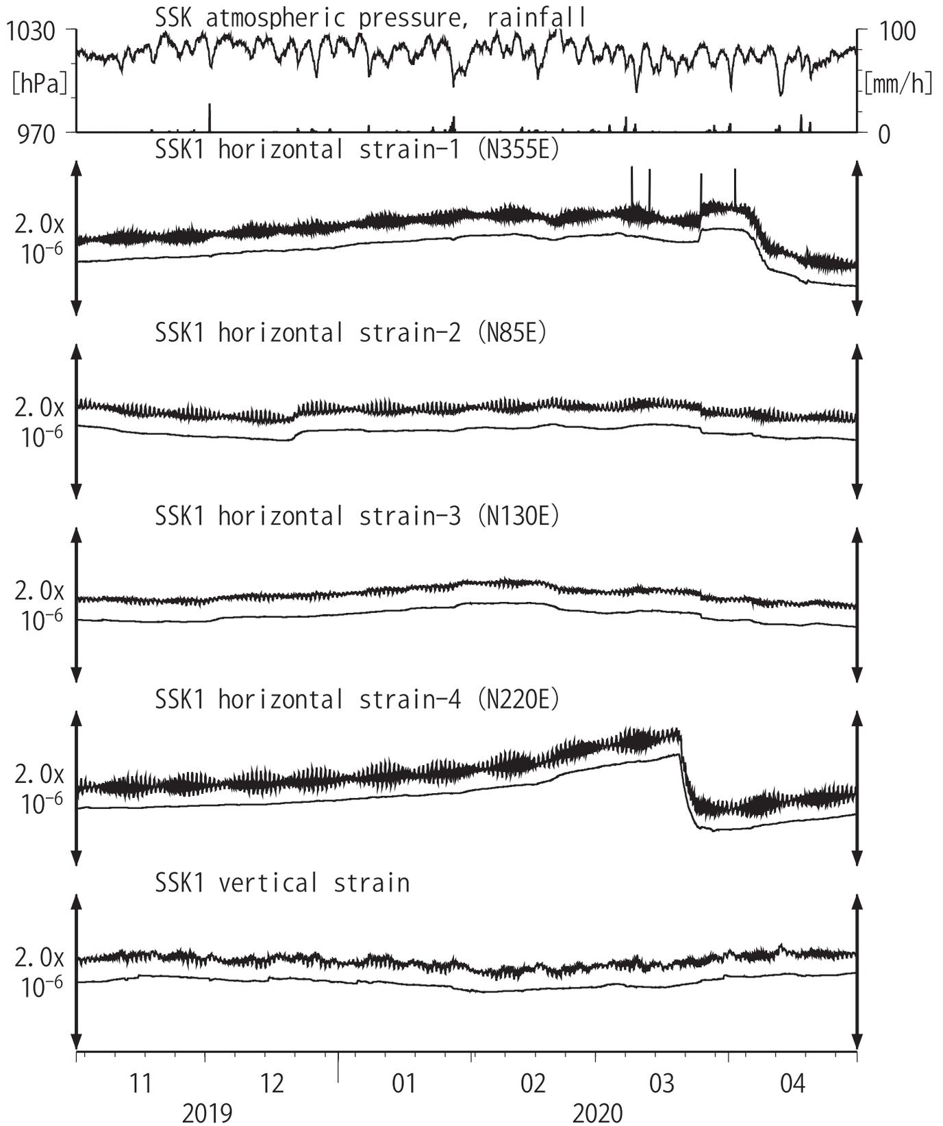
Strainmeter depth = 576.7-578.1 [GL-m]
