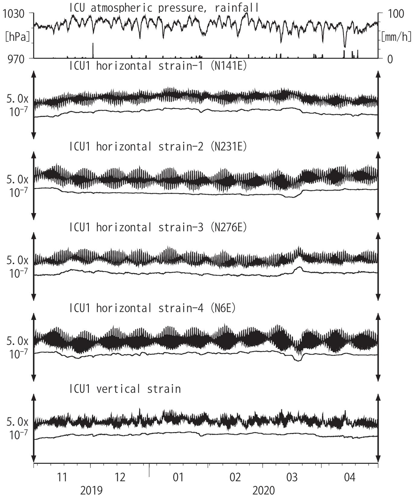
Strainmeter depth = 588.5-589.9 [GL-m]
