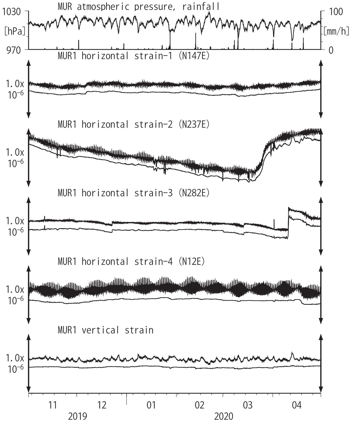
Strainmeter depth = 587.5-588.9 [GL-m]
