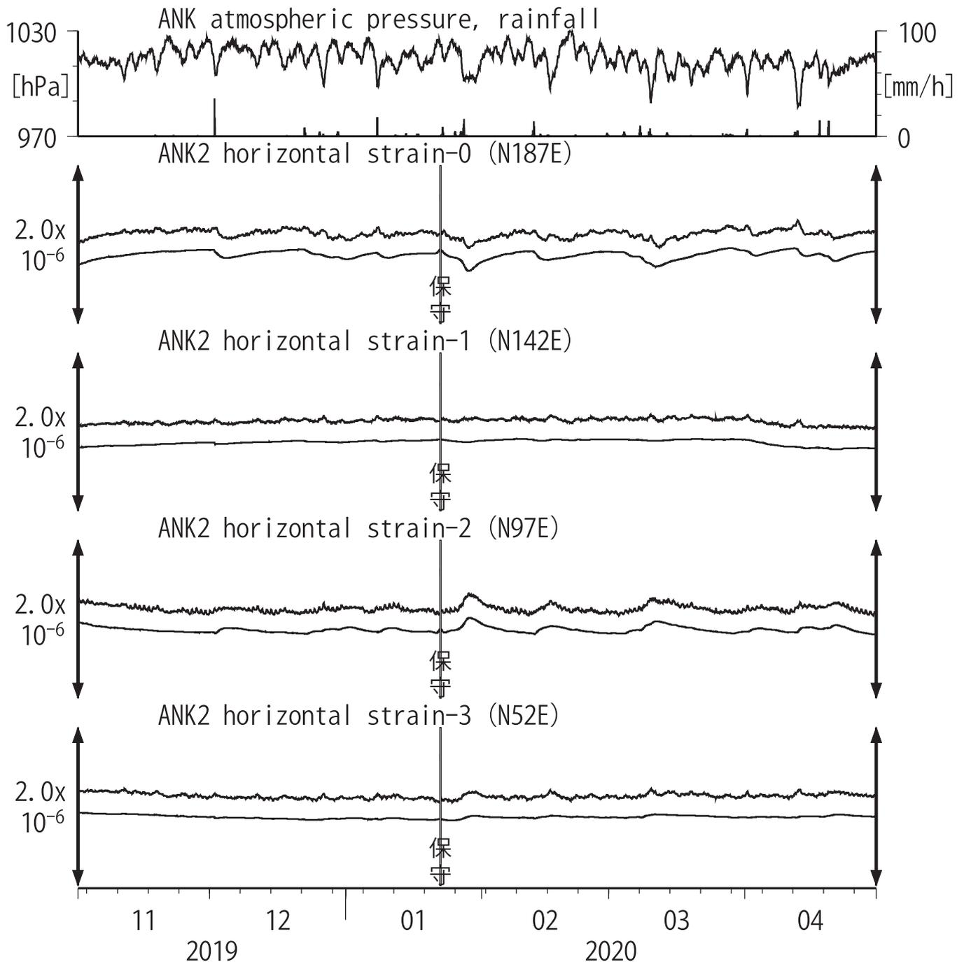
Strainmeter depth = 166.0-168.3 [GL-m]
