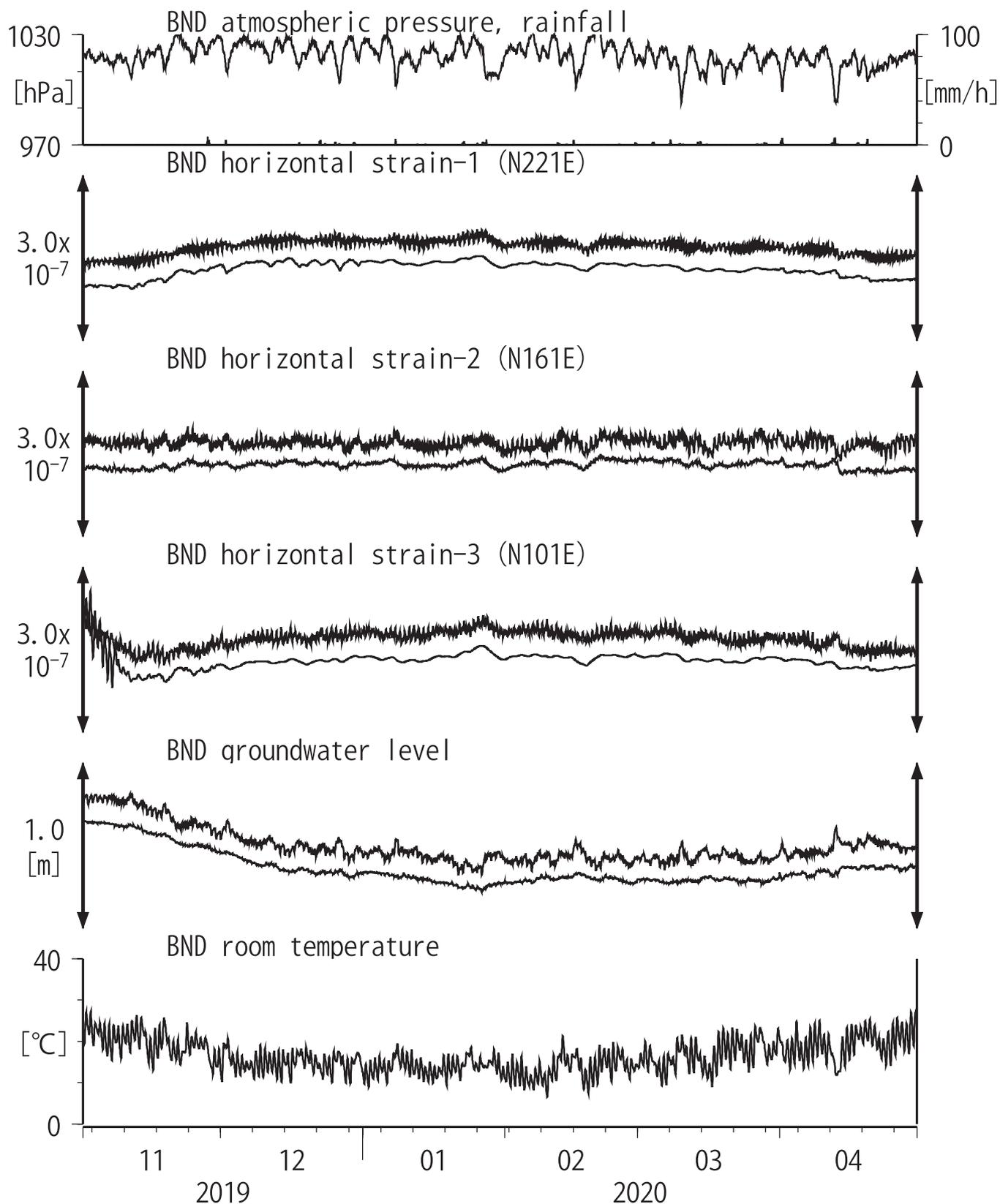
Strainmeter depth = 496.5-496.7 [GL-m]
