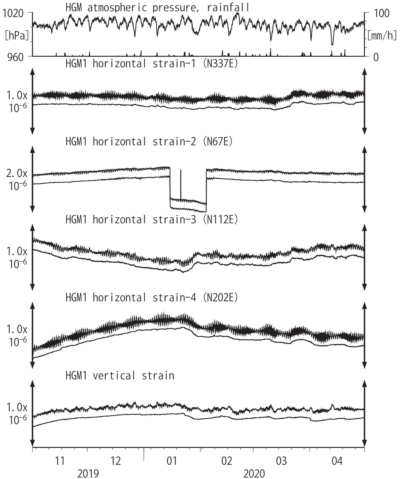
Strainmeter depth = 372.7-374.1 [GL-m]
