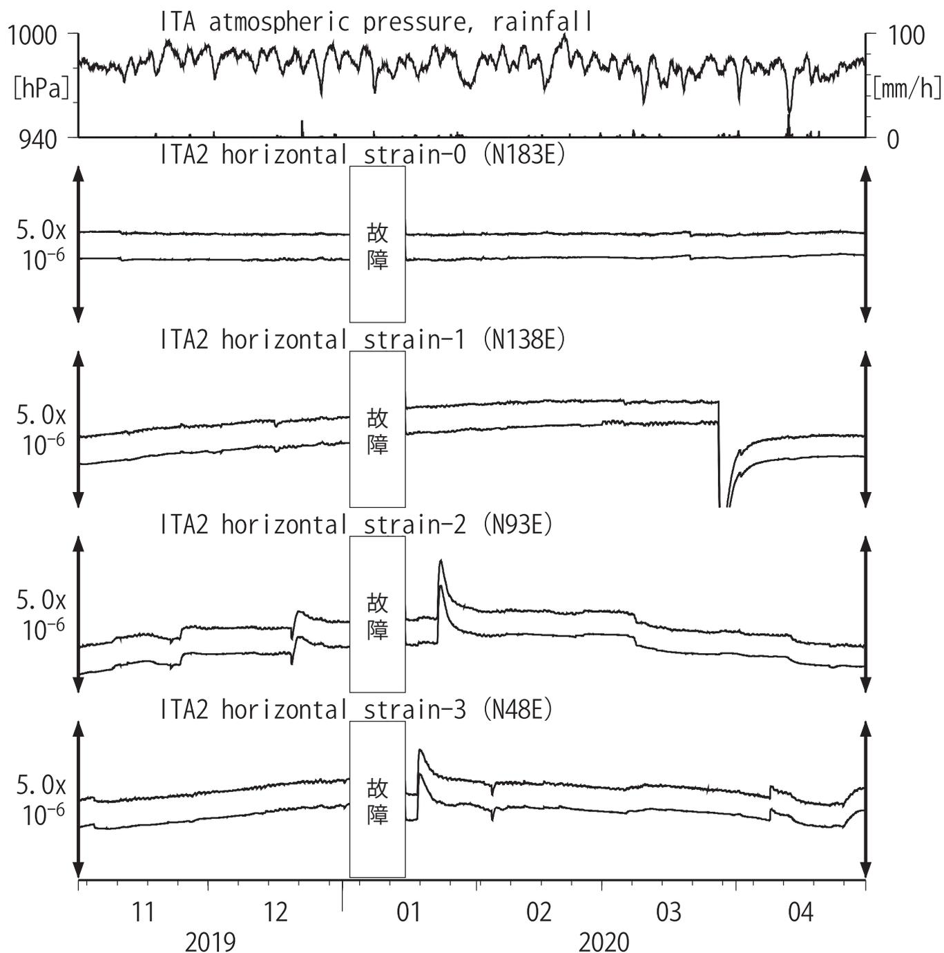
Strainmeter depth = 181.3-183.6 [GL-m]
