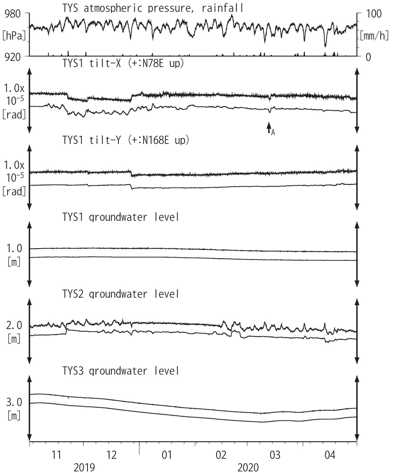
Tiltmeter depth = 585.9-586.7 [GL-m]
