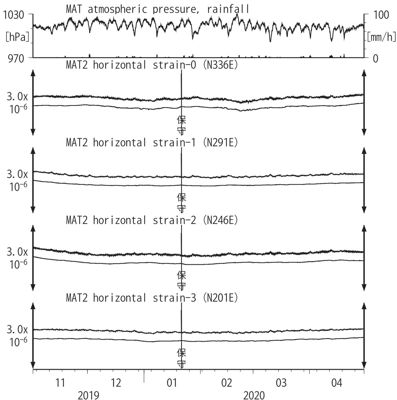
Strainmeter depth = 200.8-203.1 [GL-m]
