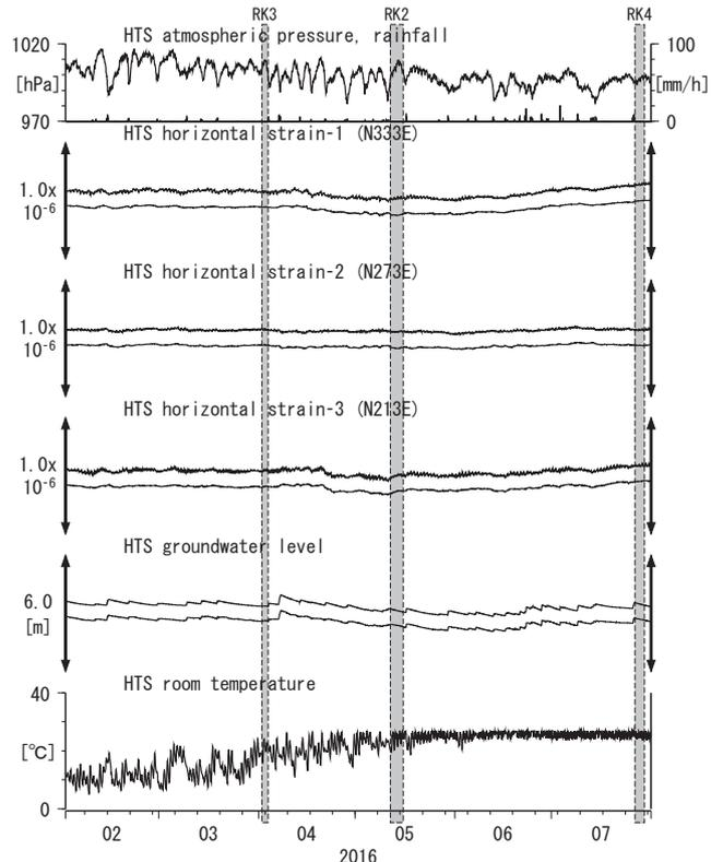
Strainmeter depth = 435.0-435.2 [GL-m]
