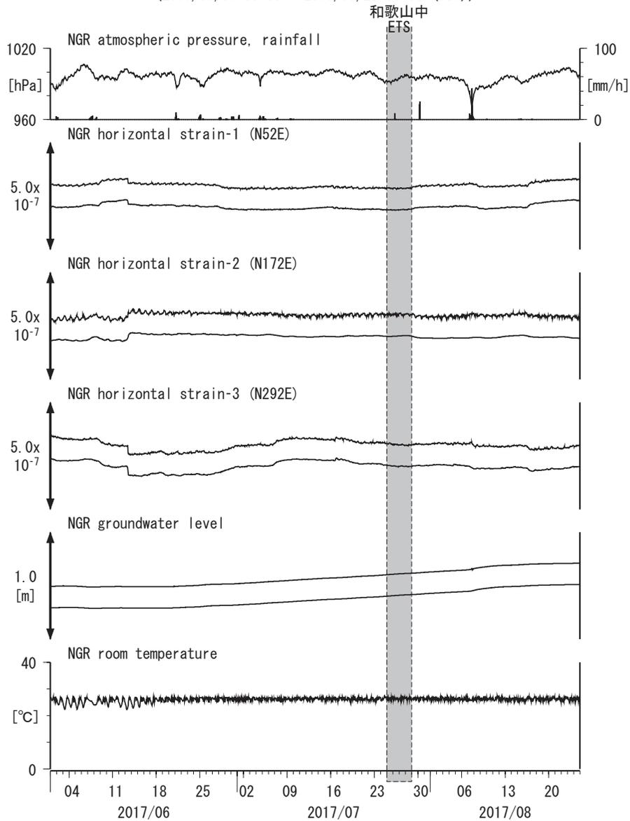
Strainmeter depth = 614.5-614.7 [GL-m]
