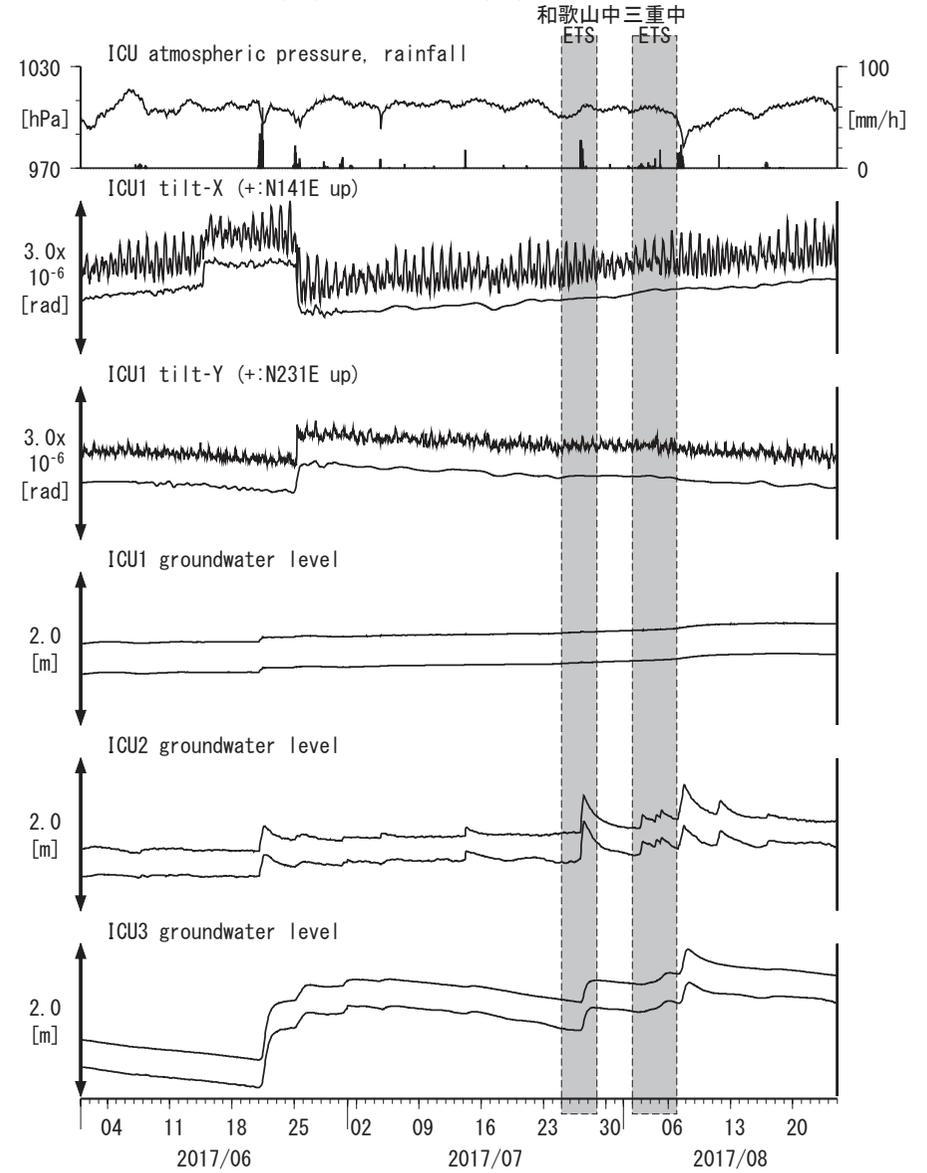
Tiltmeter depth = 587.7-588.5 [GL-m]
