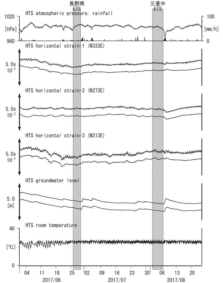
Strainmeter depth = 435.0-436.2 [GL-m]
