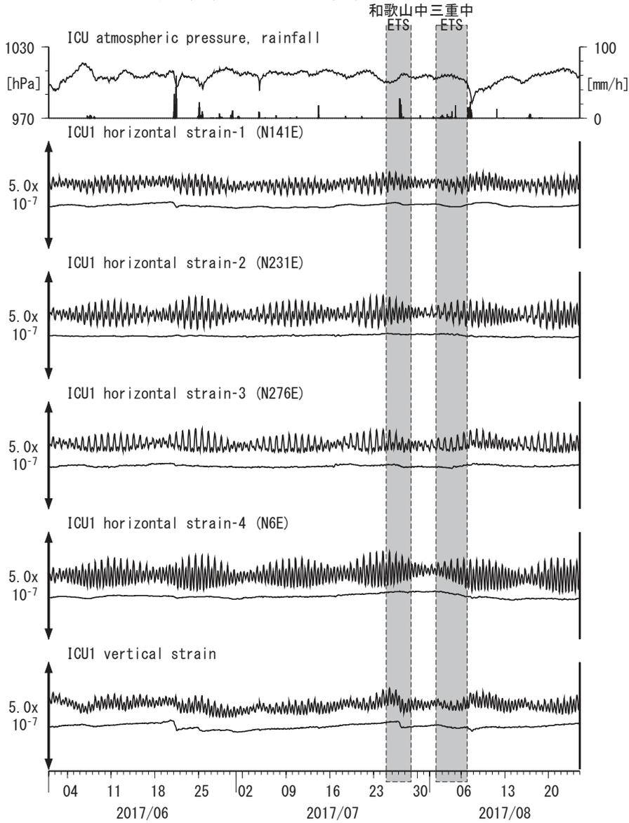
Strainmeter depth = 588.5-589.9 [GL-m]
