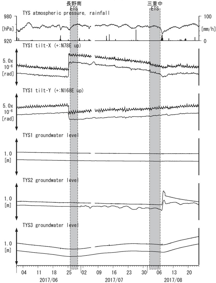
Tiltmeter depth = 585.9-586.7 [GL-m]
