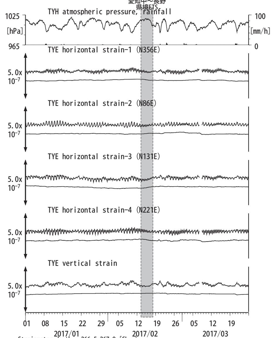
Strainmeter depth = 266.5-267.9 [GL-m]
