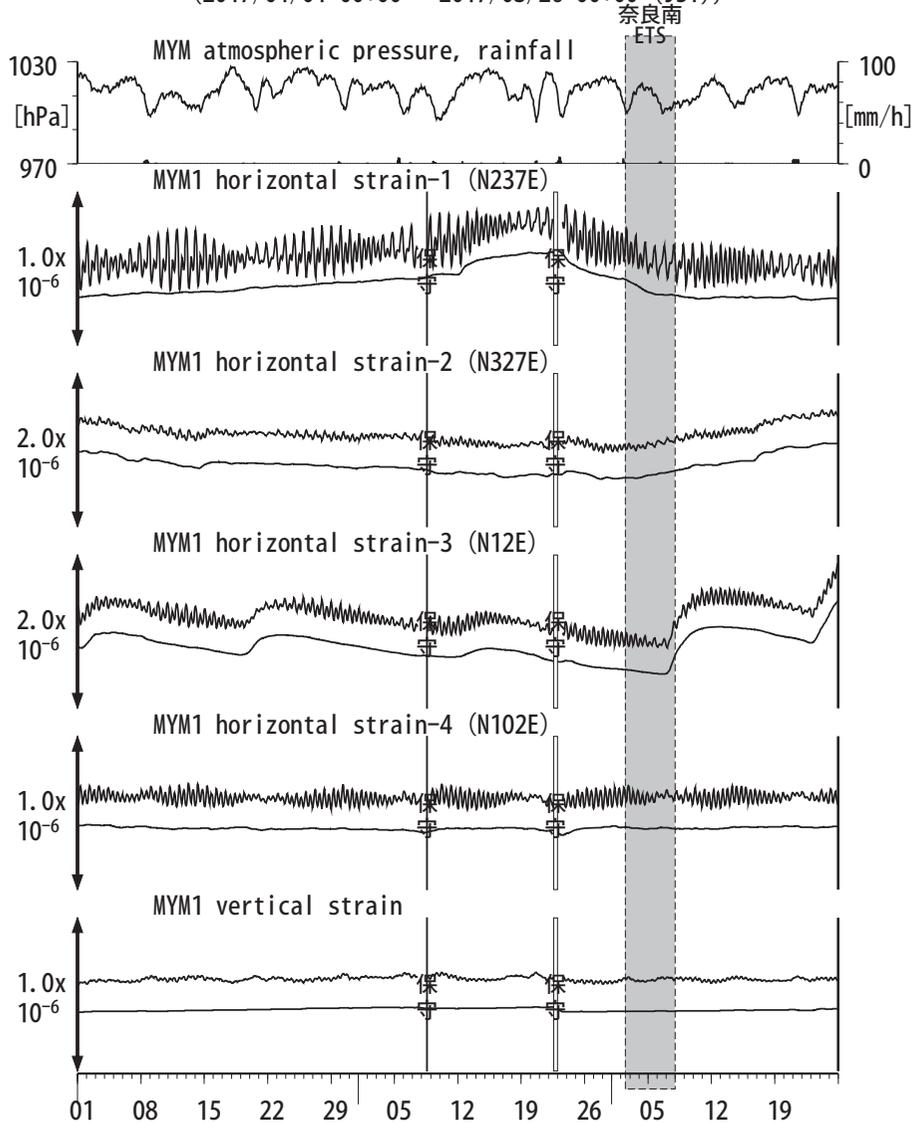
Strainmeter depth = 590.0-591.4 [GL-m]
