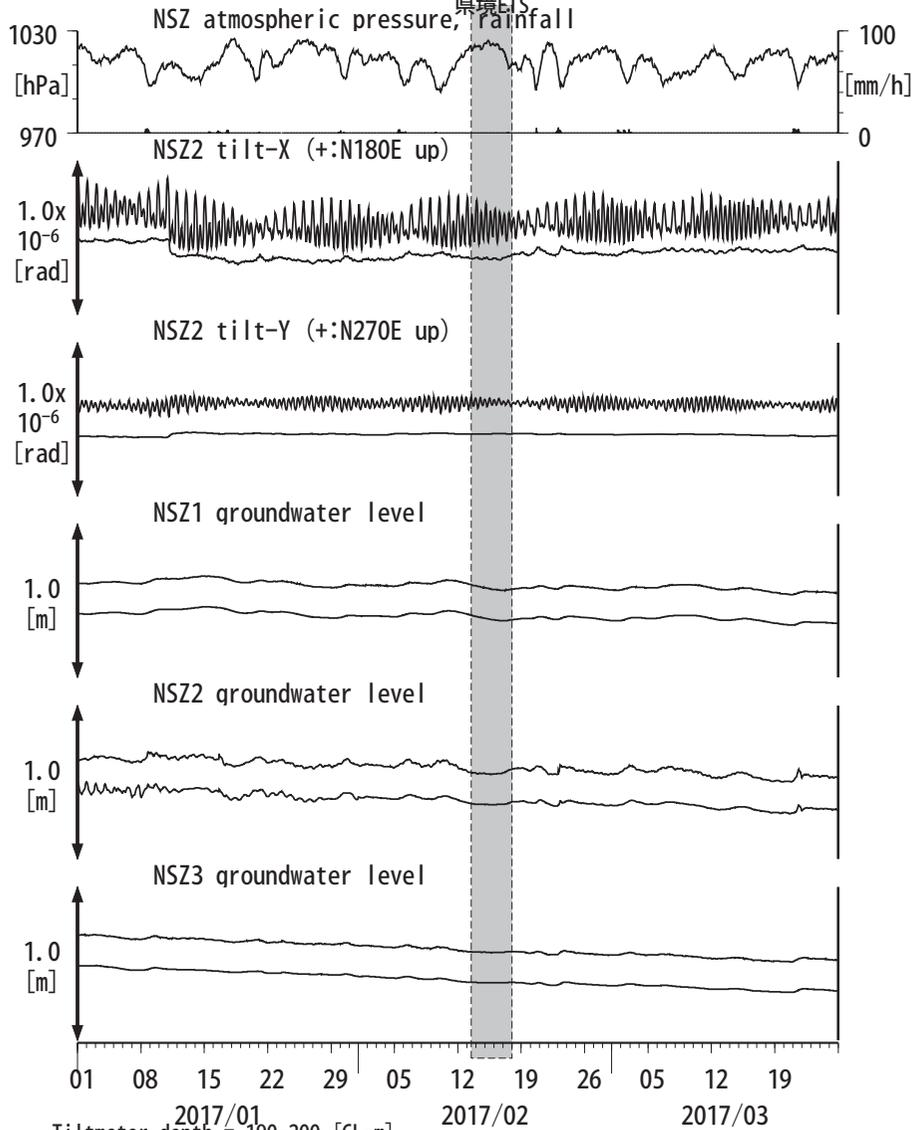
Tiltmeter depth = 190-200 [GL-m]
