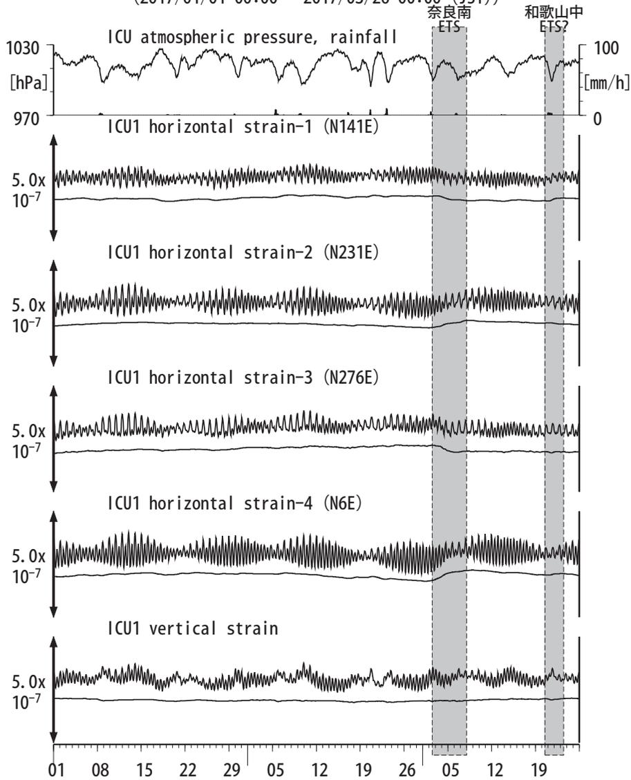
Strainmeter depth = 588.5-589.9 [GL-m]
