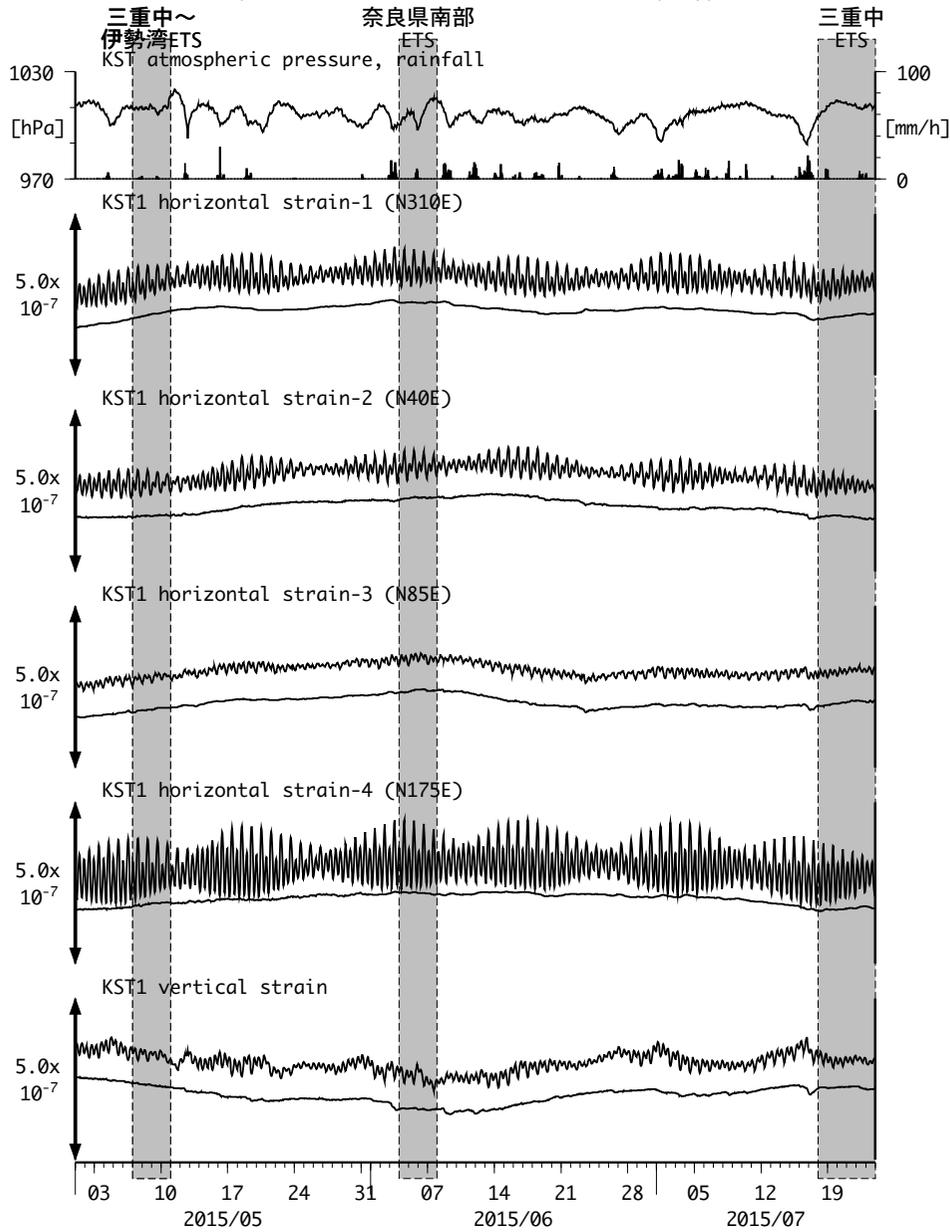
Strainmeter depth = 589.8-591.2 [GL-m]
