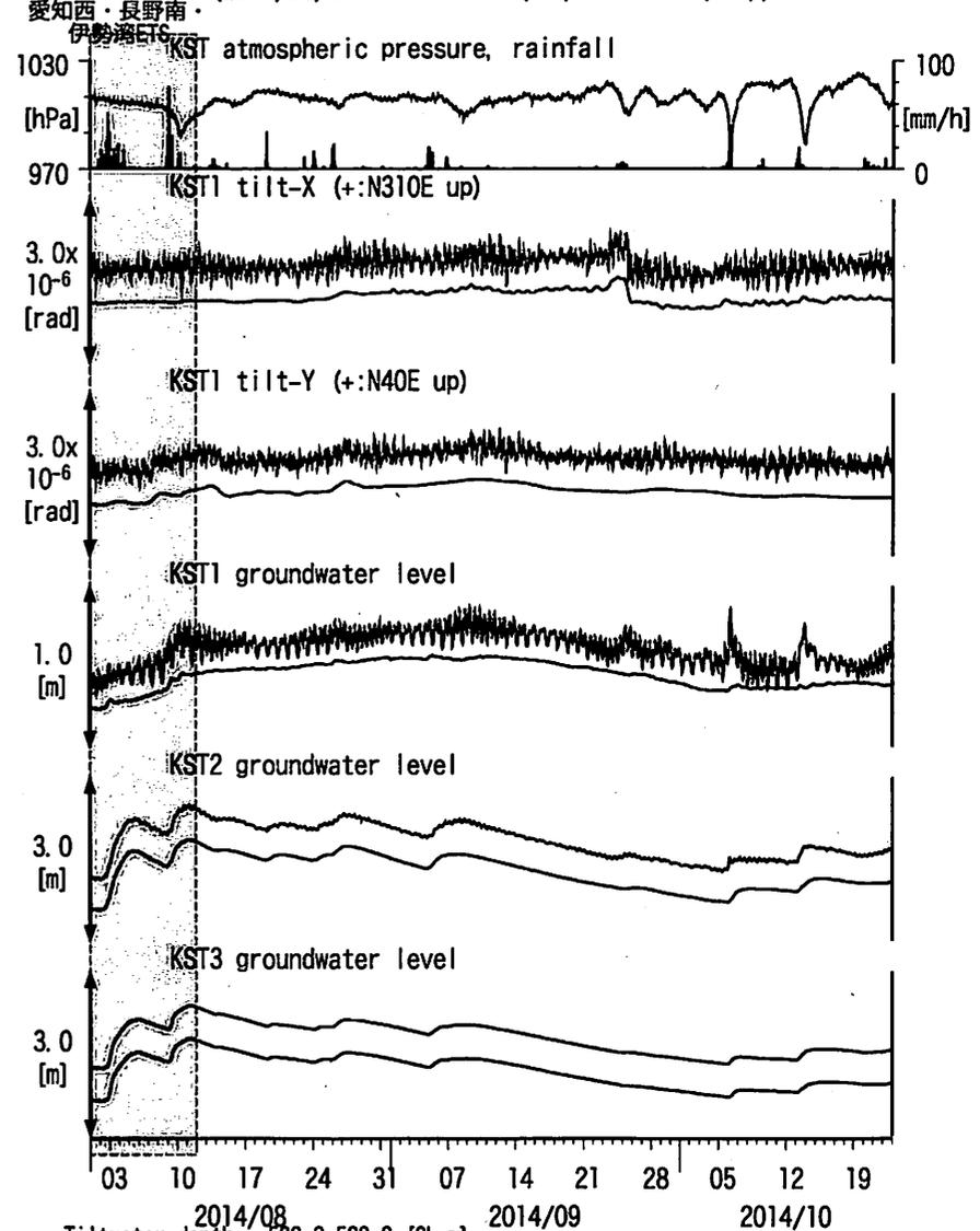
Tiltmeter depth = 589.0-589.8 [GL-m]
