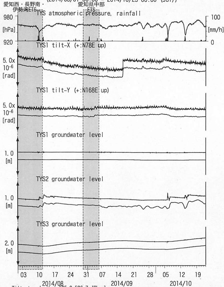
Tiltmeter depth = 585.9-586.7 [GL-m]
