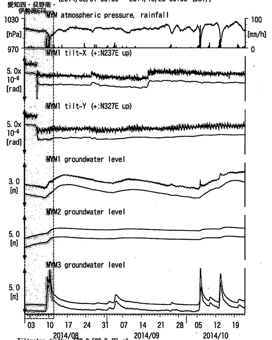
Tiltmeter depth = 589.2-590.0 [GL-m]
