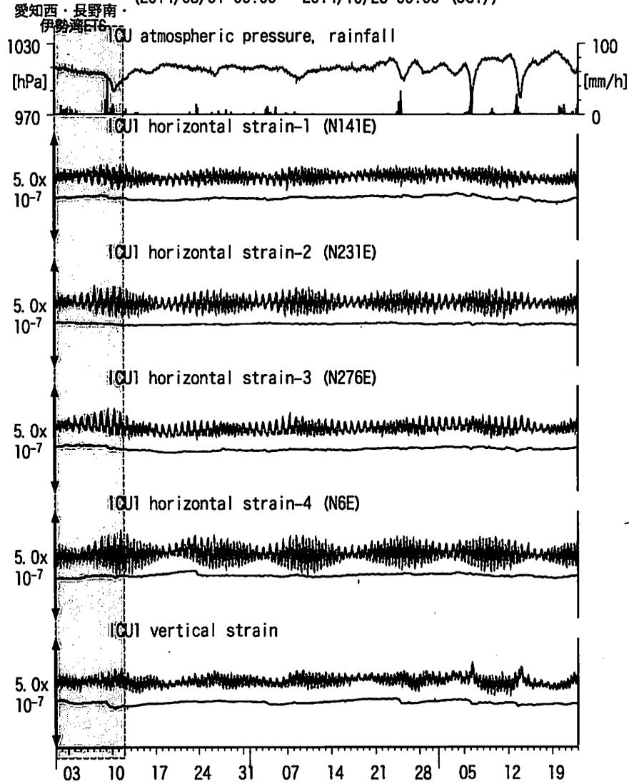
Strainmeter depth = 588.5-589.9 [GL-m]
