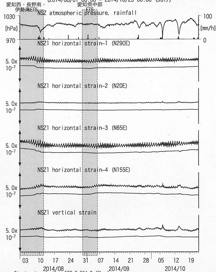
Strainmeter depth = 582.3-584.3 [GL-m]
