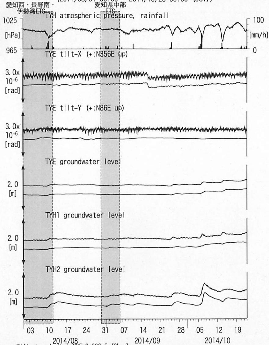
Tiltmeter depth = 265.6-266.5 [GL-m]
