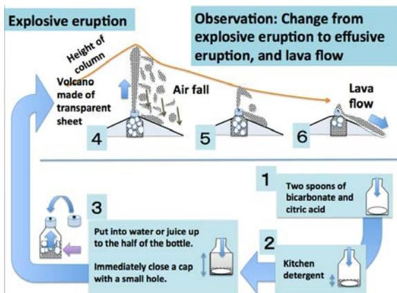
Fig.3. Experimental procedure of explosive eruption.
