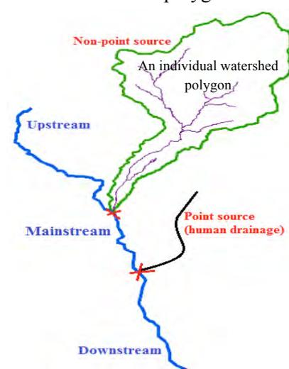
**Fig. 1.** Conceptual model of an individual non-point contaminant source zone
