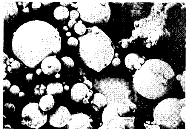
Fig. 3d Surface of the Naile fly ash in SEM
