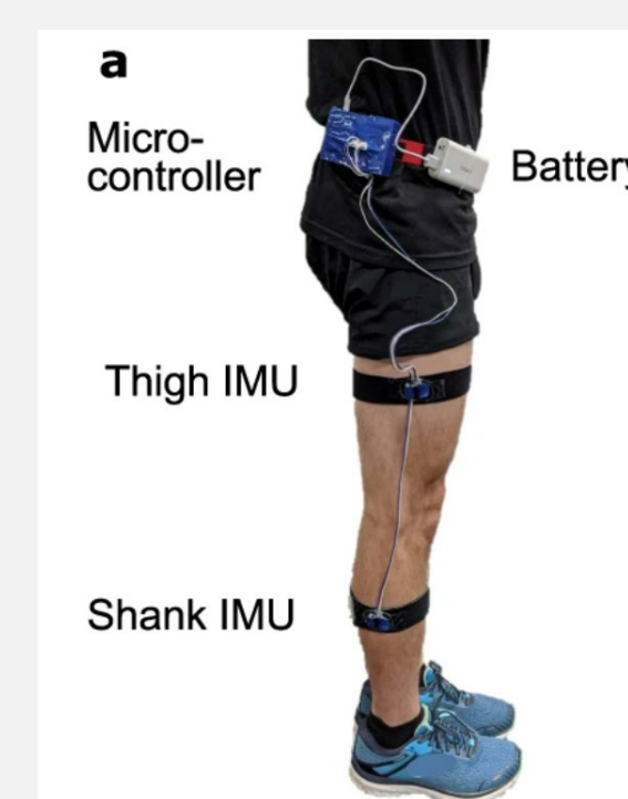
Fig.9: (Wearable) OpenMetabolics: Schematic and hardware prototype
