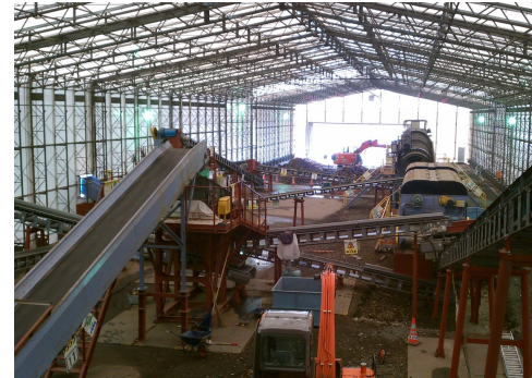
Advanced separation at secondary temporary storage sites 二次仮置き場での高度選別
