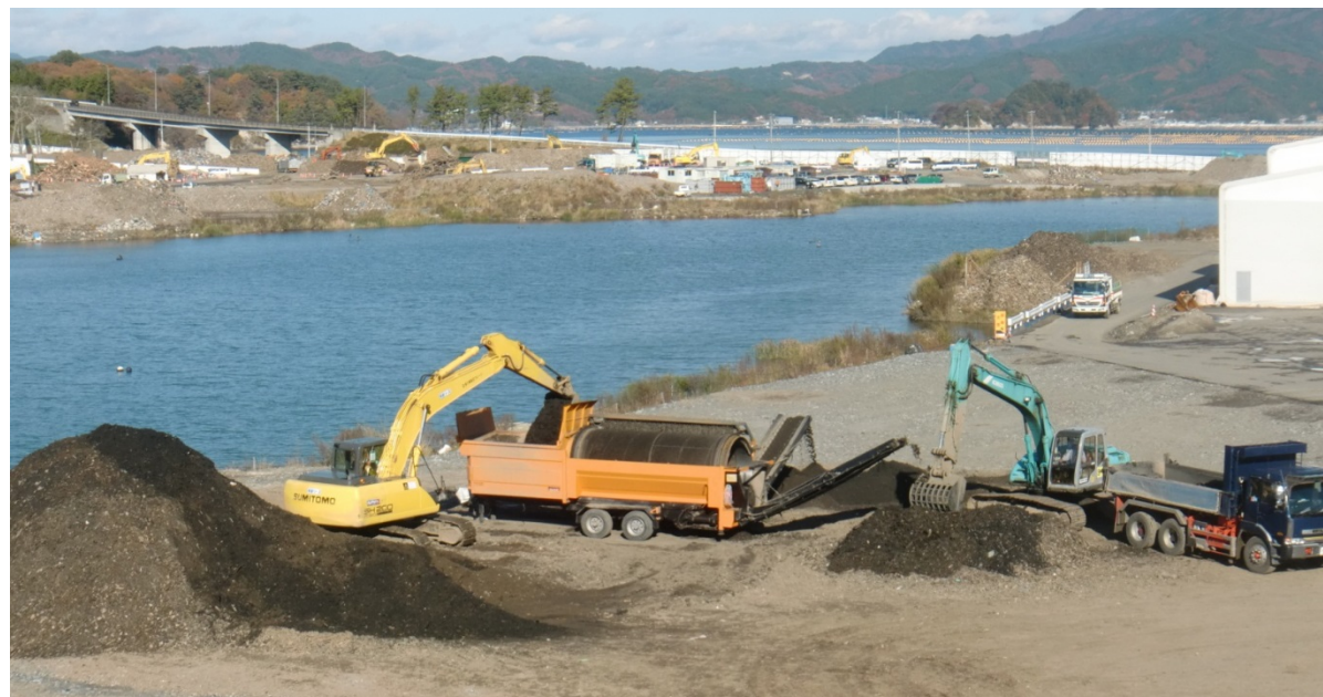
Separation from soil-dominant stockpiles (Yamada town) 土砂系混合物(津波堆積物)の分別
