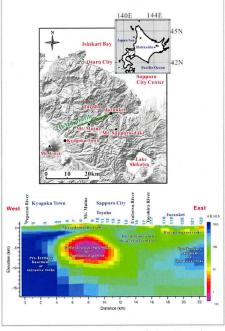
A 2-D resistivity section of the Toyoha geothermal area, including Mt. Muine and the Jozankei hot springs as analyzed and interpreted for the 2D profile.
