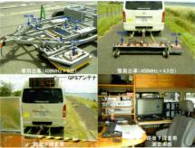
Truck-mounted ground-penetrating radar system for the detection of soft around zones.
