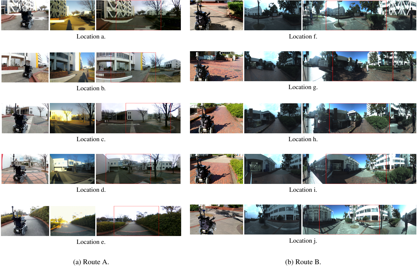
Figure 12: Navigation experiments. Left:Robot in motion. Center:Estimated location (i.e., best matched training image). Right:Input image and selected moving direction.
