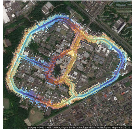
Fig. 7. Mapping result by LiTAMIN for the big loop case. The background aerial photograph is referred to Google Map.
