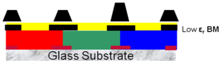
Figure : CF on TFT Array Design (Black Matrix and R/G/B layers are moved to TFT substrate side.)
